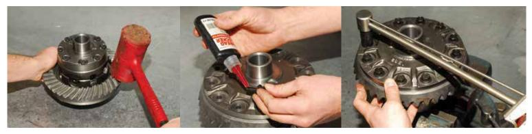
2. Install Bearing races in housing and press Pinion & Carrier Bearings. Make sure to keep track of the position & size of any shims, baffles, or slingers if/where applicable.
